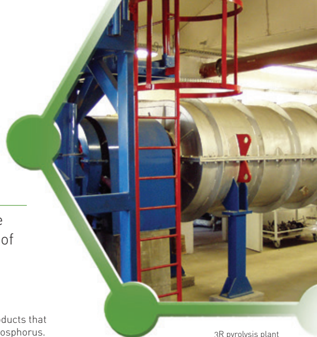
3R pyrolysis plant
